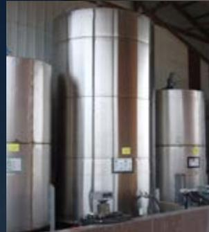
Liquid bins go through a wash and treatment system to remove any particles that may be left on the surface, followed by back welding interior seams and are then pressure tested. Liquid fittings are added to these bins making the handling of liquid products trouble free.
