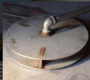
The AirMix is a pulsating air injection system across the bottom of the tank. Operators can select the speeds and settings of the pulsing action with Meridian's Variable Control System, changing the duration and the frequency of the air agitation within the tank. Gentle
