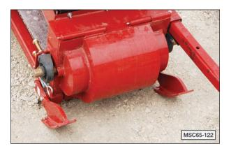
9. If removed, reinstall the discharge hood.
