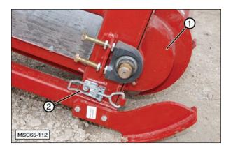
3. The belt should track in the middle of the top and bottom rollers, as shown.
