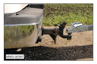
5. If equipped, place the jack in its stowed position.
