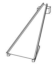
3. Temporary storage can be provided by erecting a simple framework supporting a waterproof tarp
