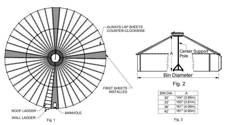
6. Caulk and place sealing foams between the roof flange and the top part of roof sheets. Sealing caps also must be inserted under sheet ribs at roof eave. At this point, assembly of the roof is completed. Securely tighten all bolts and make sure roof is completely watertight.
