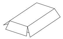
4. All bin boxes, ladder boxes and hardware boxes should be stored inside. These are not waterproof, and will deteriorate in normal weather conditions, allowing moisture to contact the parts inside.
